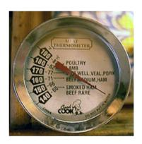
Meat Thermometer - A thermometer used to measure the internal temperature of meat, especially roasts and steaks, and other cooked foods. The degree of "doneness" of meat correlates closely with the internal temperature, so that a thermometer reading indicates when it is cooked as desired.
