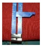
**Sewing Gauge** — A short ruler that has a moveable slide for marking hems, seams, and other areas.
