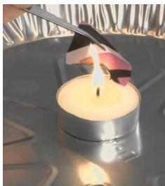
**Test Procedure:** Select small sample of at least six to eight yarns about 4 inches long and twist them together into about a 1/8 inch bundle or use a small square of your fabric. Hold one end with tweezers over a protected fire-resistant surface. Use a candle or match for flame.
